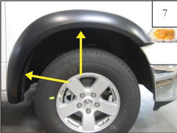
Hold flare to vehicle and start supplied #8x3/4" Washer Panhead Screws with a Phillips screwdriver. *Do not tighten.*
